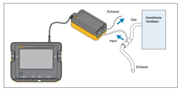
Figure 4. Anesthesia Gas Connections
