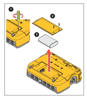
Figure 5. Battery Replacement
