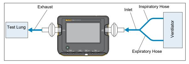
Figure 1. Bi-Direction Flow Mode Connections
