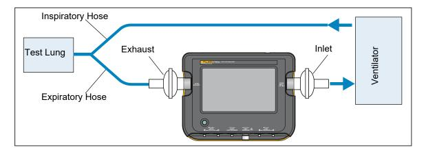
Figure 3. Expiratory Breathing Circuit Connections
