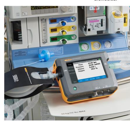
Onboard memory and USB for easy data transfer and test file upload to your CMMS 7" (17.8 cm) color touchscreen showing real-time graphs and test data. Allows for customizable test profiles (by user, test type, or model) and data logging
