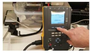
B. Press the "test" button and wait. The red isolation test light will illuminate on the ESA.
