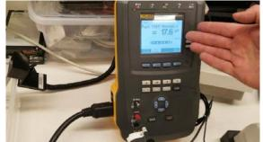
It is our recommendation that you record your results and compare them to future tests in regularly scheduled intervals. Over time, the leakage of the ultrasound may increase as the insulation of the probe breaks down due to use and cleaning. A proactive service and repair schedule should protect against the probe failing and causing a down time event.
