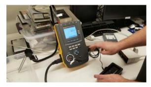
B. Connect the second 3476233 adapter to the red "V/ $\Omega$ /A" Port. Plug the ultrasound specific adapter plate into the adapter.
