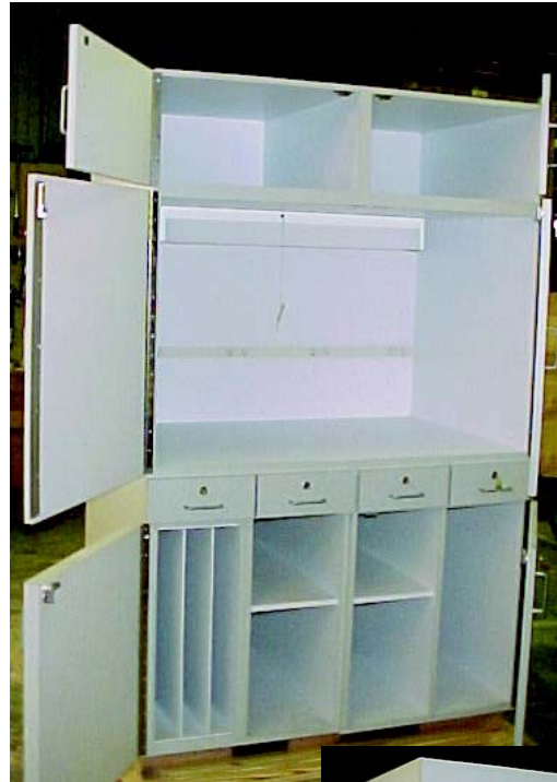
Stand-alone workstation with 0.13 inch lead on all surfaces and 0.75 inch leaded flood phantom storage compartment
