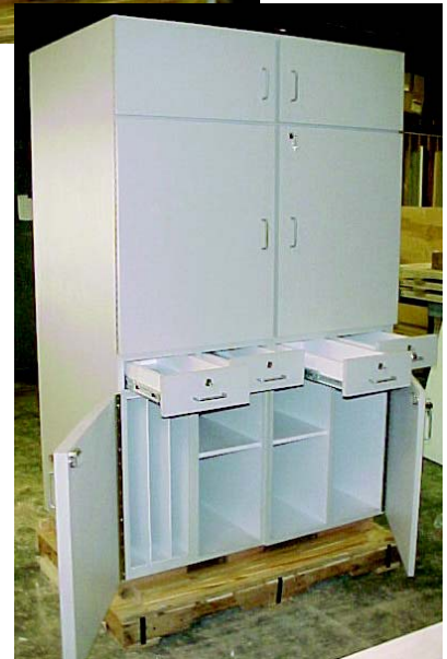
Stand-alone workstation with 0.13 inch lead on all surfaces and 0.75 inch leaded flood phantom storage compartment
