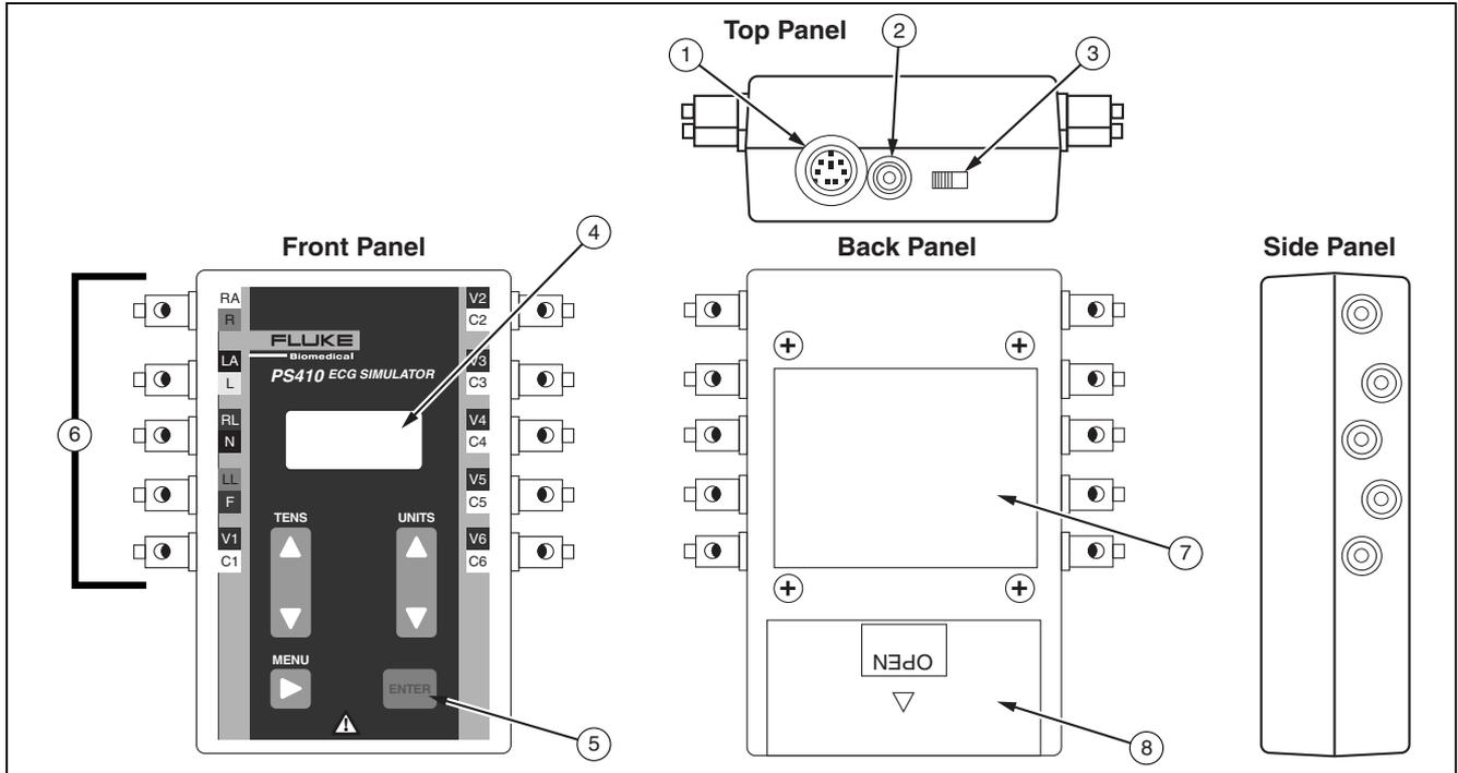
**Figure 1. Controls and Terminals**
