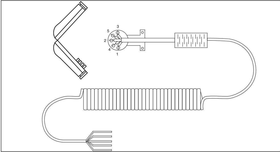
**Figure 3-1. Unterminated Blood Pressure Output Cable Assembly**
