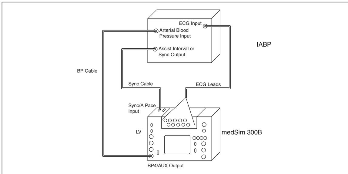
Figure 4-24. Connections for Intra-Aortic Balloon Pump (IABP) Simulation
