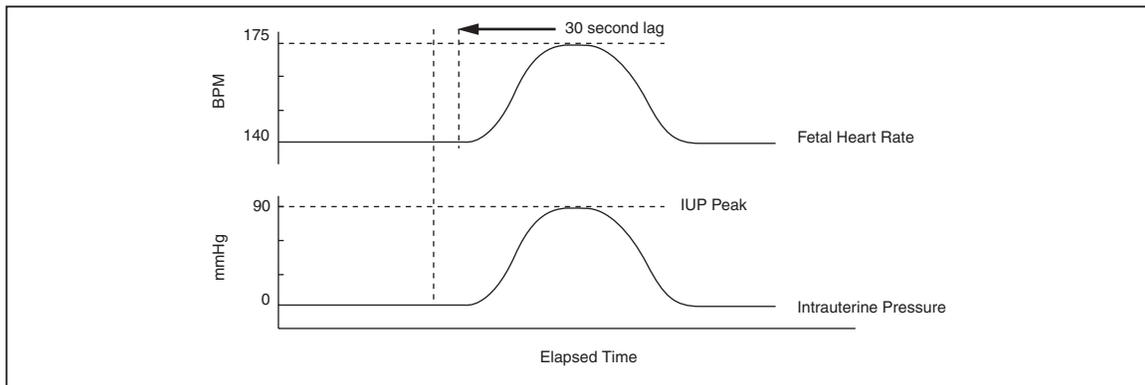
**Figure 4-22. medSim 300B Simulated Uniform Acceleration**
