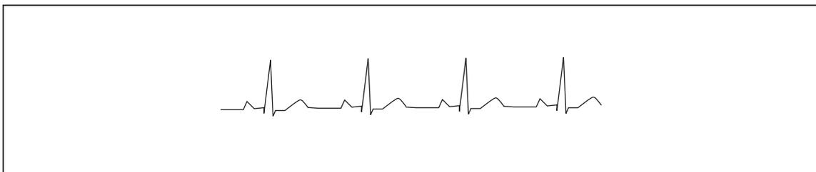
**Figure 4-16. medSim 300B Simulated Maternal ECG**
