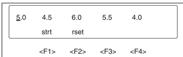
2. One of the segments (in this case, 5.0) has a cursor under it. Press <F1>-STRT to execute the marked segment. Upon execution, the marked segment (5.0) starts flashing, and the cursor marks the next segment (4.5).
