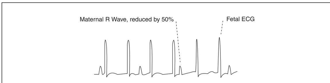
**Figure 4-17. medSim 300B Simulated Maternal ECG with Fetal ECG Added**
