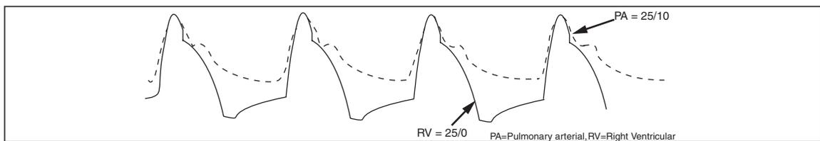
Figure 4-3. medSim 300B Simulated Waveforms for Normal Blood Pressure Relationships across the Pulmonary Valve
