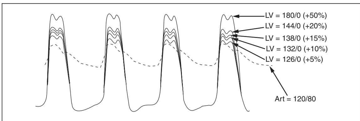
Figure 4-2. medSim 300B Simulated Systolic Pressure Gradients Indicating a Defective Aortic Valve
