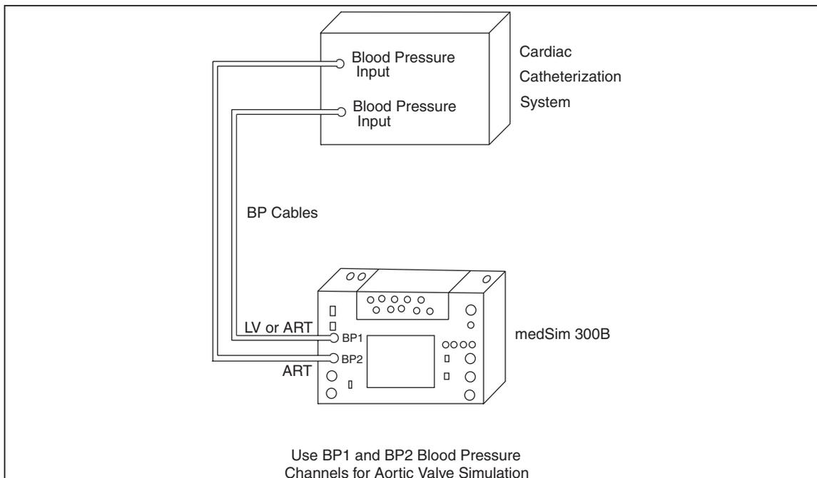
**Figure 4-5. Cardiac Catheterization Connections for Aortic Valve Simulation**
