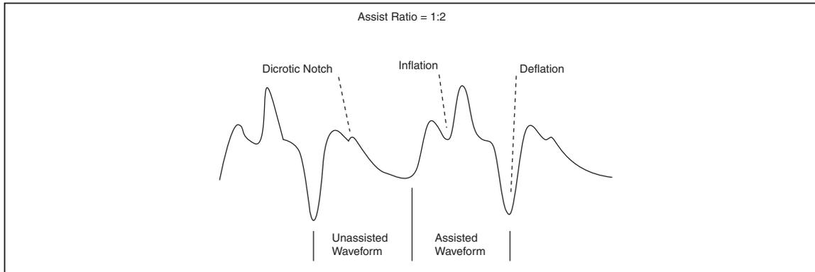
**Figure 4-25. medSim 300B Simulated Normal Waveform with the IABP Properly Set**
