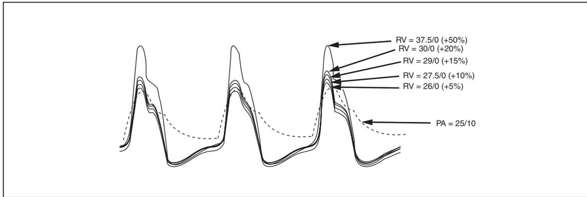
**Figure 4-4. medSim 300B Simulated Systolic Pressure Gradients Indicating a Defective Pulmonary Valve**
