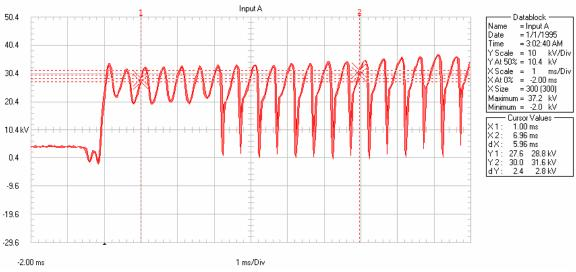
This is the capture of a set of microspits, minor tube arcs. These were captured at 48 KV with no scope offset before the exposure.
