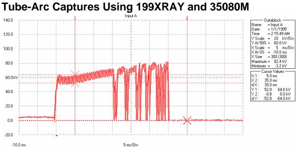
This is a classic tube arc, captured just before the circuit breaker tripped. This was captured using Fluke Biomedical's 199XRAY Medical ScopeMeter used in conjunction with the 35080M non-invasive kVp Divider. Notice the KV gradients on the left side of the image. This is a very powerful tool.
