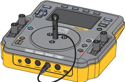
A yellow and grey incubator analyzer with an air flow sensor inserted into the top port. A cable connects the sensor to the front panel port labeled 'AIR FLOW'. <p data-bbox="1398 904 1469 918">hxy006.eps</p> |
