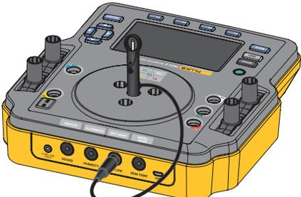
A yellow and grey incubator analyzer with an air flow probe inserted into the top circular port. A black cable is connected to the front panel. <p data-bbox="1398 905 1469 918">hxy006.eps</p> |
