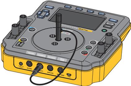
A yellow and grey incubator analyzer with a humidity probe inserted into the top circular port. A black cable connects the probe to the front panel port labeled 'HUMIDITY'. <p data-bbox="1398 552 1469 565">hxy004.eps</p>  |
