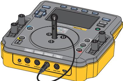
A yellow and grey incubator analyzer with an air flow probe inserted into the top circular port. A black cable connects the probe to the front panel port labeled 'AIR FLOW'. <p data-bbox="1398 901 1469 915">hxy006.eps</p> |
