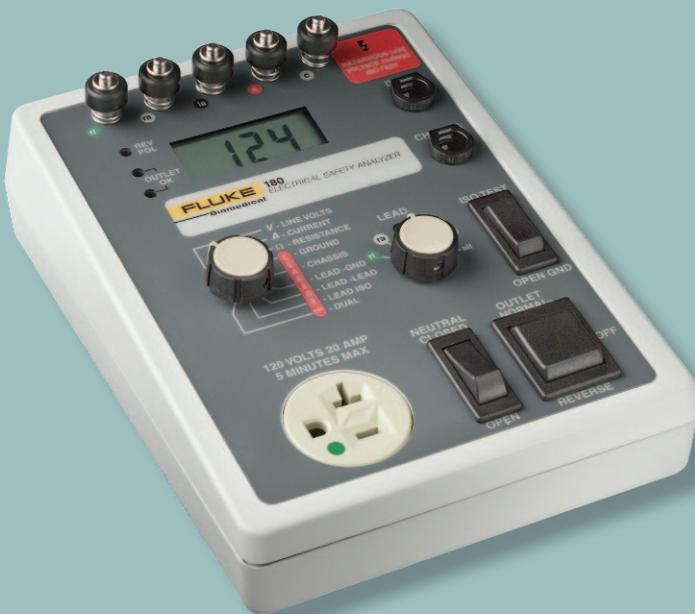
The handheld 180 Electrical Safety Analyzer is a lightweight, portable device for testing electrical systems, medical devices, and physiological instrumentation. The device includes the AAMI test load and has 5 jacks for patient applied parts testing.
