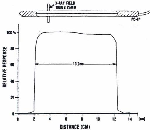
Fig 2. Chamber response to narrow x-ray.
