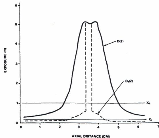
Fig 5. Exposure profiles for scans using no sleeve,  $[D(Z)]$ , and a sleeve with  $A > 0$ ,  $[D_1(Z)]$ .
