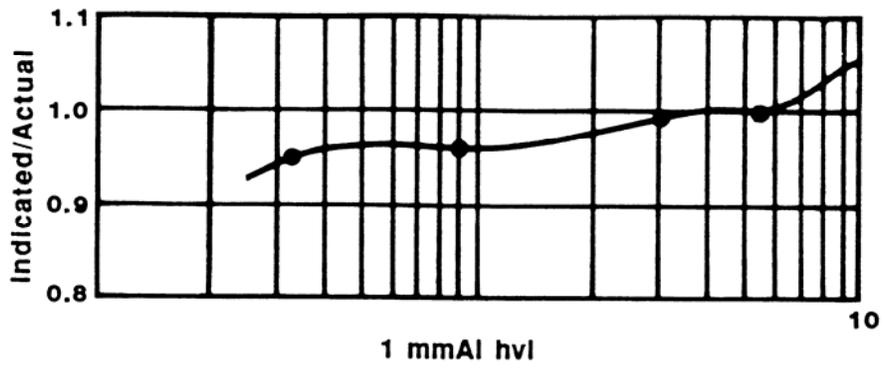
Figure 1-3. CT Probe Energy Response (Phantom Adapter Removed)
