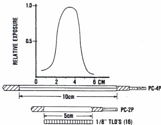
Fig 3. Comparison of single exposure profile to active length of detector systems.
