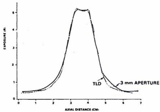
Fig 7. Exposure profile for TLD's and for a sleeved probe for  $A=3 \text{ mm}$  calculated using Eq. (12). The parameters are  $A = 0.3 \text{ cm}$ ,  $B = 0.013$ ,  $L = 10.2 \text{ cm}$  and  $X_0 = 1.24 R$ .
