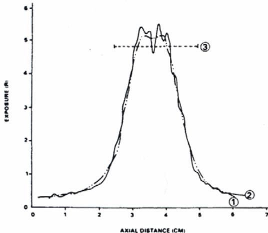
Fig 6. Exposure profiles for 3 cases; 1) TLD's spaced as intervals of 0.9 mm, 2) TLD's spaced at 3.2 mm intervals, and 3) with  $X(t) = X_0 L t^{-1} = X_0 (10.2 \text{ cm}) (2.6)^{-1}$
