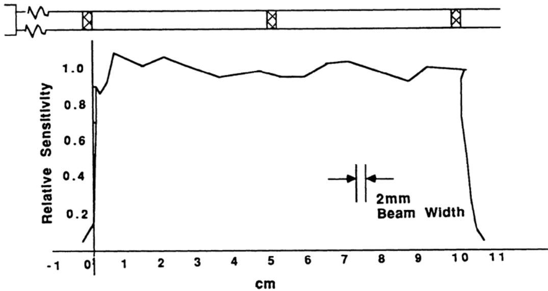
*Figure 1-4. CT Probe Unit Length Response*
