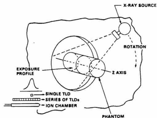
Fig. 1. Schematic of typical CT scanner operation. The axis of rotation of the x-ray tube, the exposure profile, the TLD's, and the ion chamber are all directed along the Z direction.
