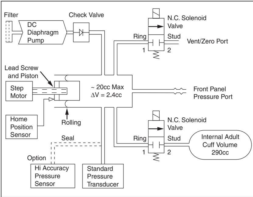
**Figure 3-1. Tester Pneumatic Block Diagram**
