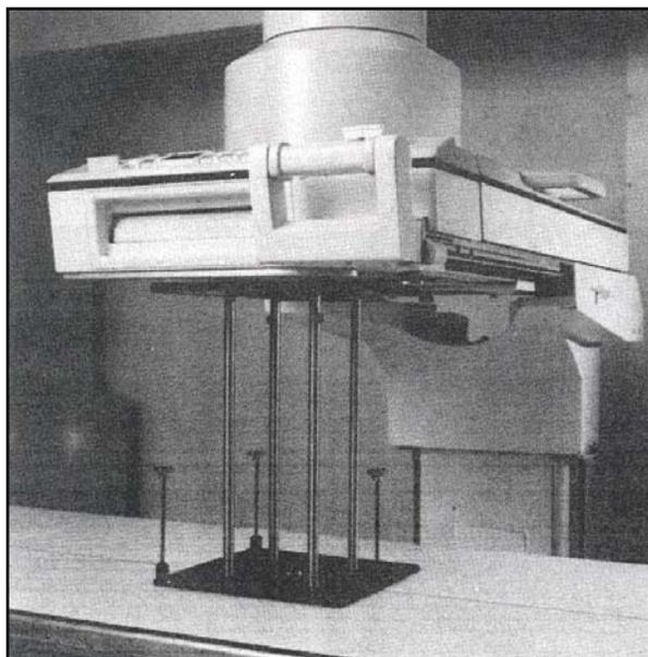
*Figure 2-7. Focal Spot Test Stand on Table (Under-Table X-Ray Tube)*
