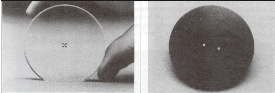
Figure 2-2. Focal Spot Test Stand Alignment Device    Figure 2-3. Magnification Insert
