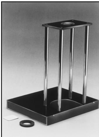
Figure 1-1. Mammography Focal Spot Test Stand (Model 07-623)
