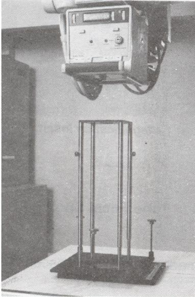
Figure 2-4. Focal Spot Test Stand Alignment Device (Over-Table X-Ray Tube)
