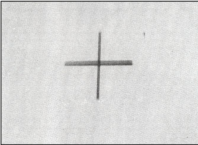
*Figure 2-8. Slit Image Parallel and Perpendicular to the Anode-Cathode Axis*
