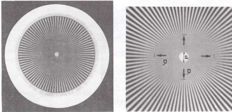
Figure 2-11. *Star Pattern Image Showing the Measurement of the Diameter of the Image of the Pattern and the Diameter at Zero Contrast.*
