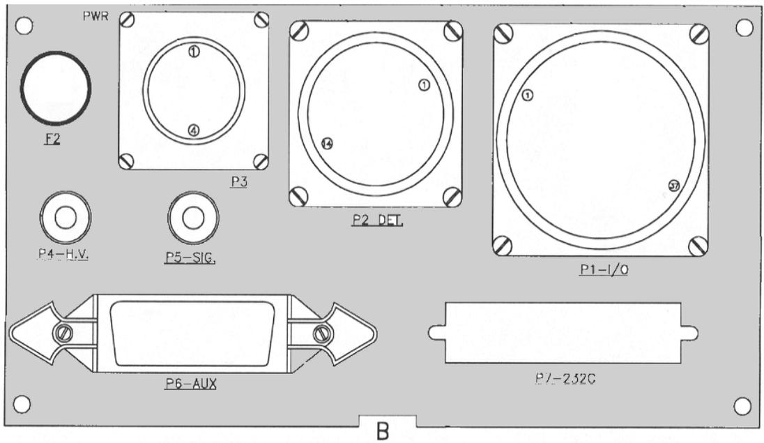
Figure 1-3. Rear Panel, Model 956A-201, Universal Digital Ratemeter (not to scale)
