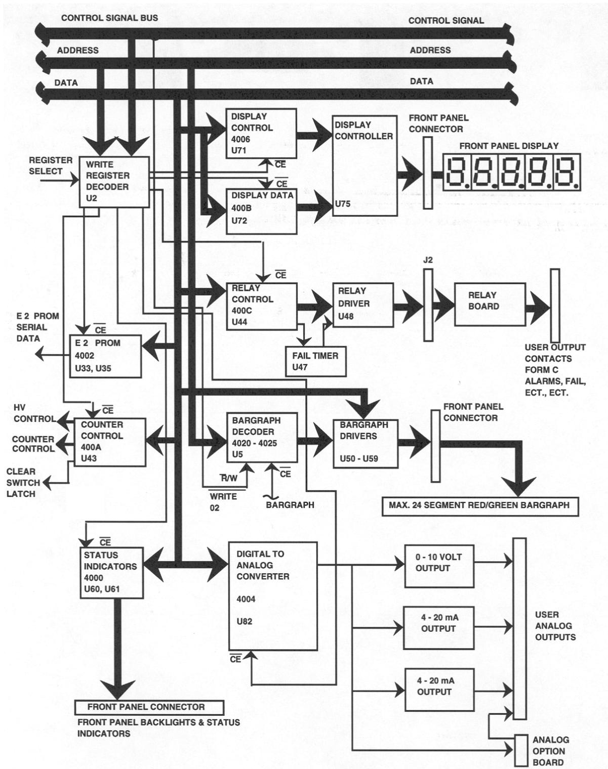
Figure 3-3. Page 2 of 3 Block Diagram – Main Circuit Board
