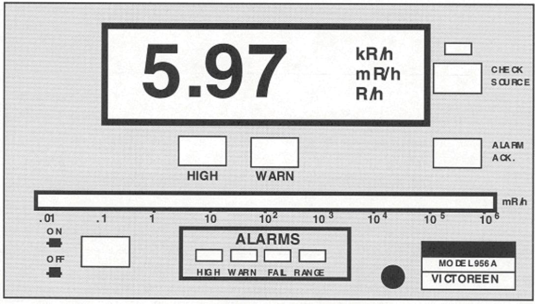
Figure 1-2. Front Panel, Model 956A-201 Universal Digital Ratemeter (not to scale)
