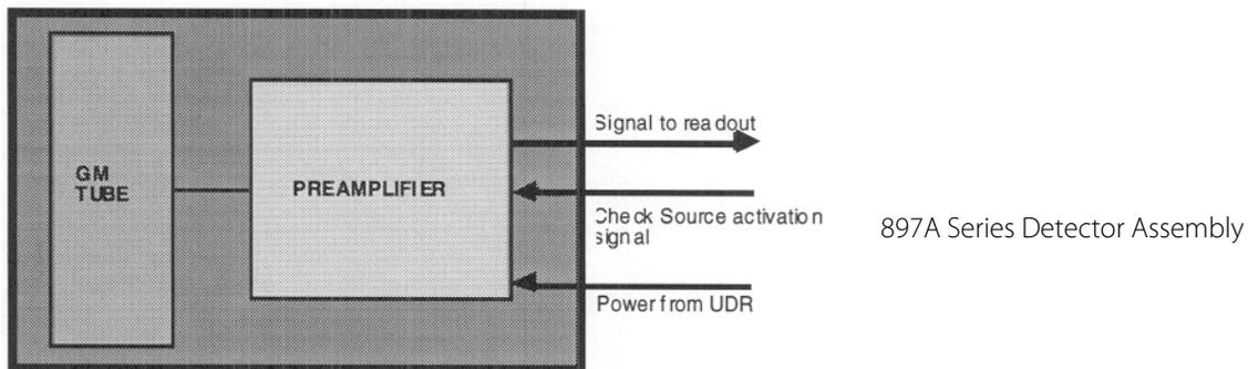
Figure 3-1. 897A Series Detector Block Diagram
