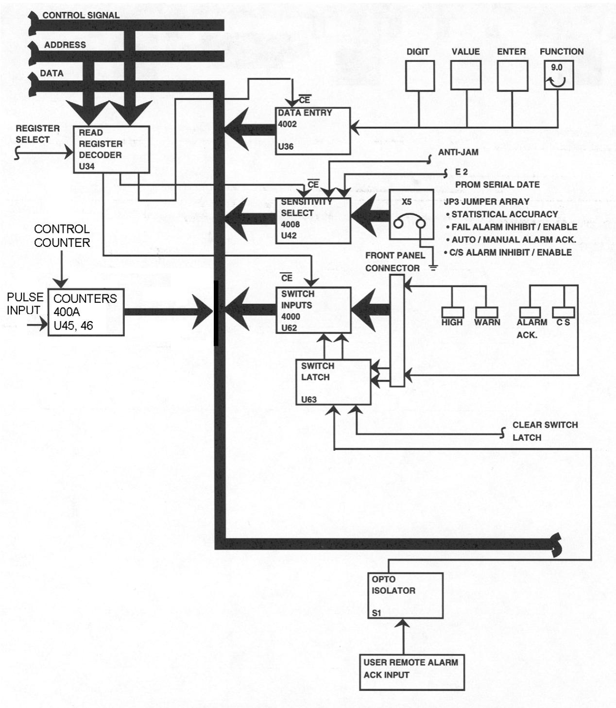
Figure 3-3. Page 3 of 3 Block Diagram – Main Circuit Board
