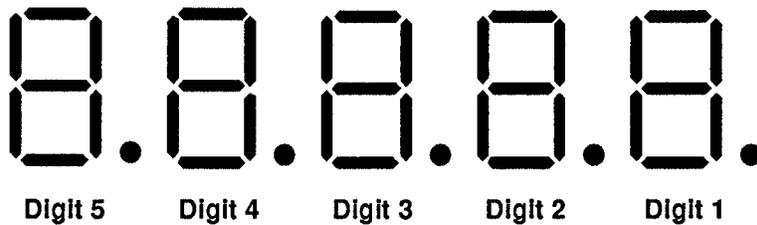
Data inputs D0-D3 and the decimal point, supplied by U72, are used to enter data in the selected digit as shown in Table 3-13.
