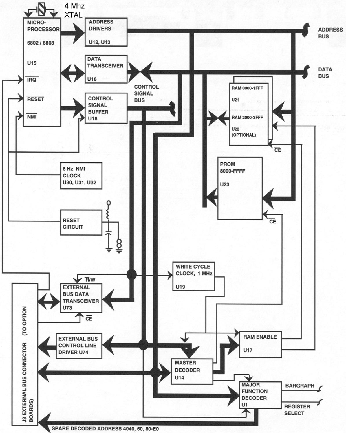
Figure 3-3. Page 1 of 3 Block Diagram – Main Circuit Board
