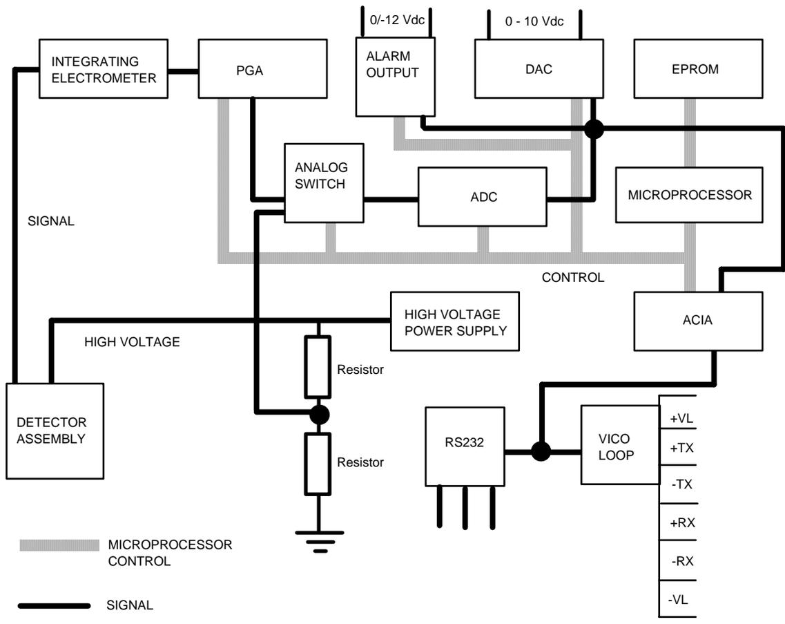
Figure 4-1. Detector Electronics Block Diagram
