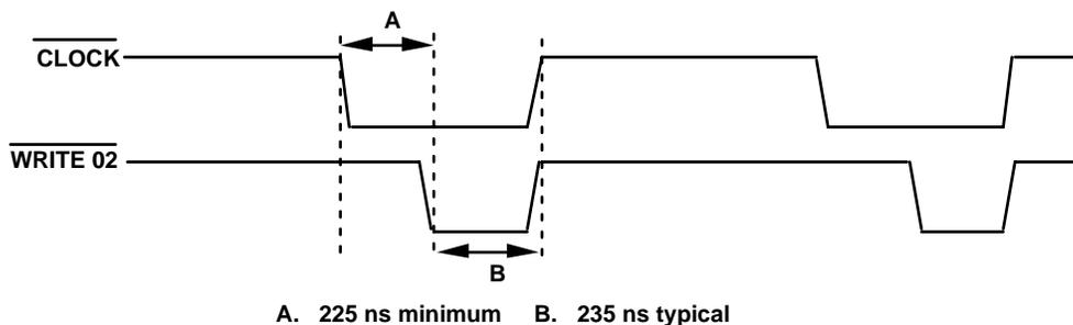
Figure 4-4. Write Cycle Clock Timing Diagram
