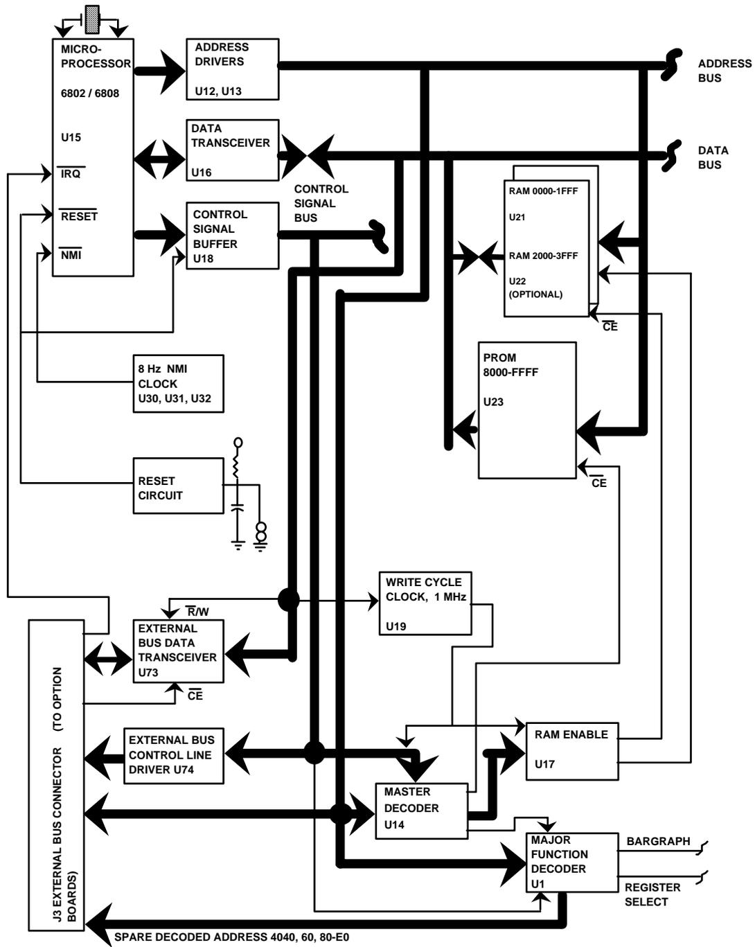
Figure 4-2. Page 1 of 3. Block Diagram - Main Circuit Board
