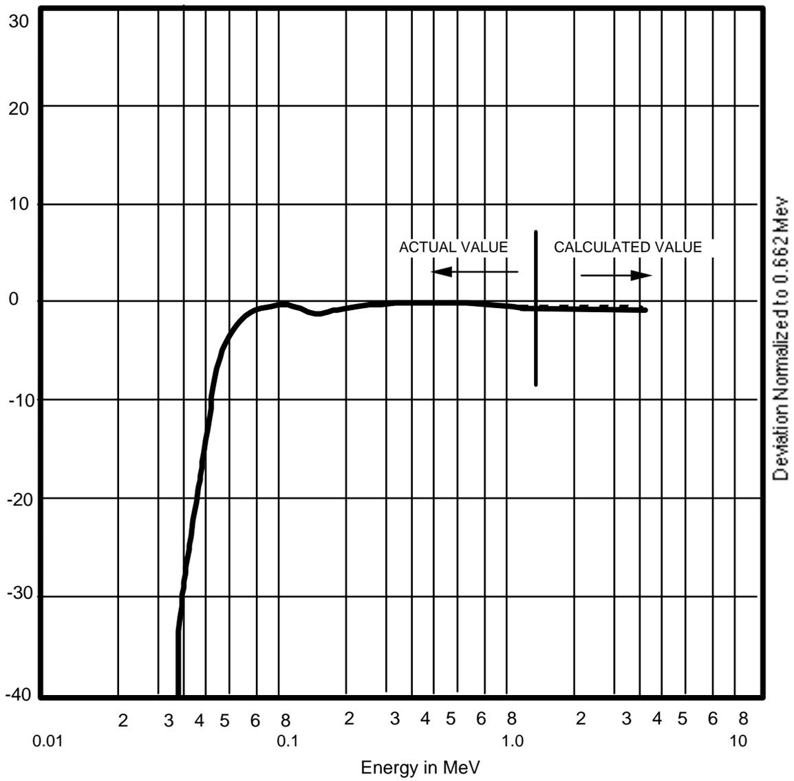
Figure 1-1. Detector Energy Response
