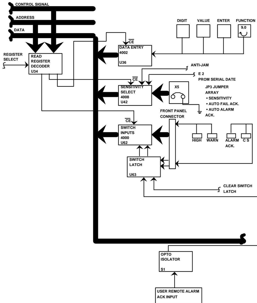
Figure 4-2. Page 3 of 3. Block Diagram - Main Circuit Board
