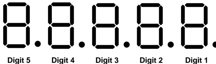
Data inputs D0-D3 and the decimal point, supplied by U72, are used to enter data in the selected digit as shown in Table 4-18.
