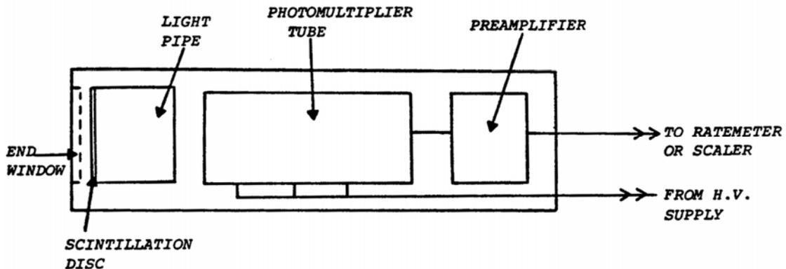
*Figure 1-1. Block Diagram, 943 Series Beta Detector*
