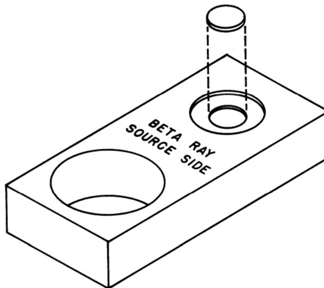
Figure 4-1. Standard Geometry Drawer Inverted to Show Recess for Beta Disk Sources
