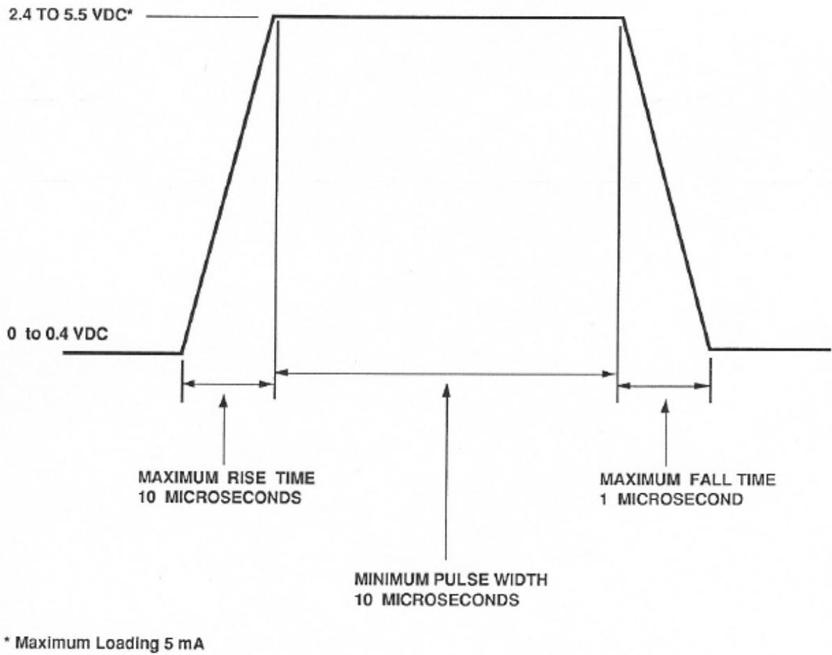
Figure 4-1. Input Pulse Specifications
