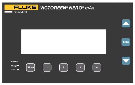
The NERO mAx display is divided into 5 columns, each column corresponds to the push button (softkey) directly beneath it. The left most column is the "MODE" column that is used to select the NERO mAx's operating mode. The remaining four columns (1 through 4) display various options for each mode.
