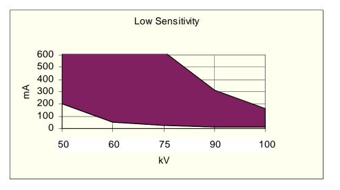
mA Limits vs. kV at 26" SDD, 1.2mm Al Inherent Filtration - Low Sensitivity:
