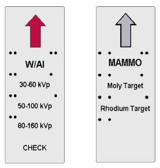
The serial numbers of the NERO mAx control console unit, detector and filter cards must be matched in order to obtain accurate results. Since the control console unit, detector and filter cards are calibrated together, they <u>must</u> be used together for accurate measurements.
