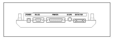
Figure 1-2. Control Console Rear Panel
