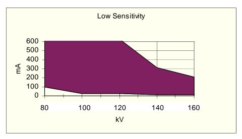
mA Limits vs. kV at 26" SDD, 1.2mm Al Inherent Filtration - Low Sensitivity: W/AI, 80 - 160 kV Filter
