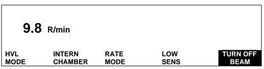
Turn off the x-ray beam. The NERO mAx has stored the measured exposure rate and will set up for the next exposure as soon as the beam turns off.
