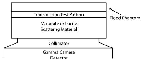
Figure 2-3. System Resolution with Scattering Material
