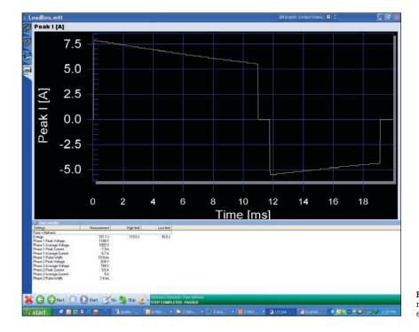
Figure 2: Defibrillator discharge curve during energy measurement test (external load 150 ohms, preset energy level 100J).
