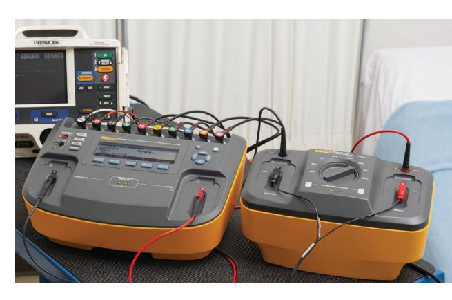
The Impulse 7010 Defibrillator Selectable Load Accessory, in conjunction with Impulse 7000 Defibrillator/External Pacer Analyzer, is specifically designed to facilitate compliance with the IEC 60601-2-4 and AAMI DF80 standards.
