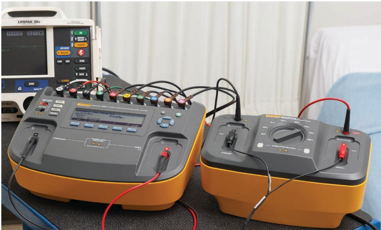
The Impulse 7010 Defibrillator Selectable Load Accessory, in conjunction with Impulse 7000 Defibrillator/External Pacer Analyzer, is specifically designed to facilitate compliance with the IEC 60601-2-4 and AAMI DF80 standards.
