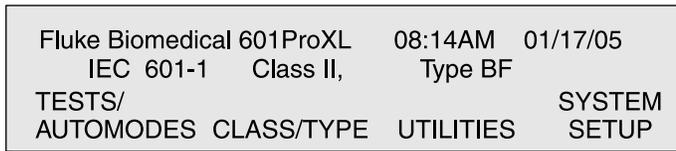
To repeat the self-check routine at any time, press **UTILITIES** from the **MAIN MENU**, then **SYSTEM TEST**.
