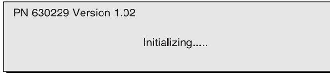
The 601PRO immediately begins a self-check routine at power-up while the following instrument identification screen is displayed:
