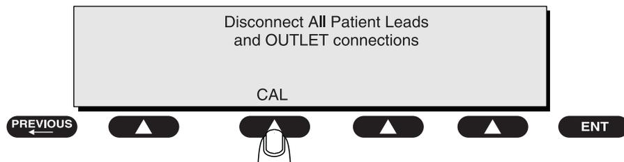
**WARNING:** *A 2-beep-per-second signal indicates high voltage present at the applied part terminals while a calibration is being performed.*
