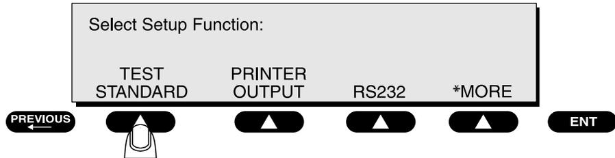
At the **Select Test Standard** menu, use one of the **SOFT KEYS** to select a test standard, or press **\*MORE** for additional options.
