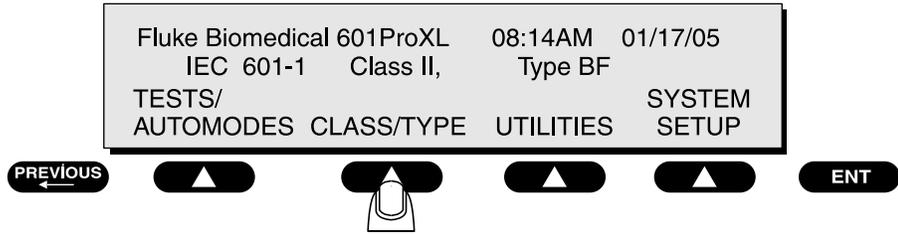
Press the **SOFT KEY** below the desired **CLASS/TYPE**, or press **\*MORE** for additional options.
