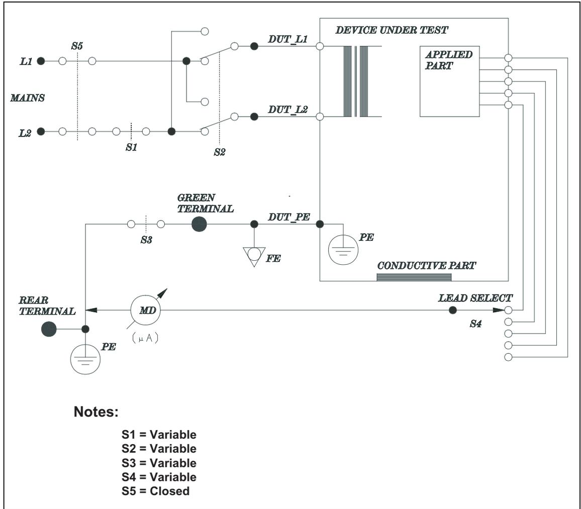
**Function:** Measures the current flowing between a selected applied part and the mains PE. The test is performed with normal and reverse mains supply polarity using S2 and single fault conditions using S3 and S1.
