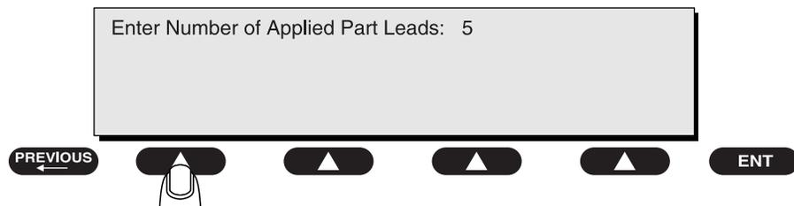
This selection allows the operator to define the number of applied parts to be tested during Mains on Applied Part, Patient Leakage, Insulation Resistance, and Patient Auxiliary Current tests. This screen will only appear when the selected Test Standard is one of the following: baw091f.eps
