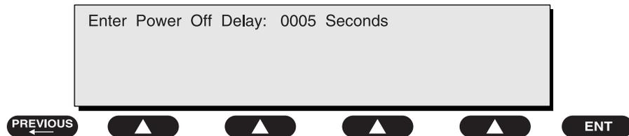
A Power Off Delay is inserted between various tests in the **Step** and **Auto** sequences. The Power Off Delay is performed after power has been removed from the DUT Outlet because the Outlet has been disabled, or L2 has been opened. A Power Off Delay allows equipment time to stop before being presented with a new power condition. baw090f.eps
