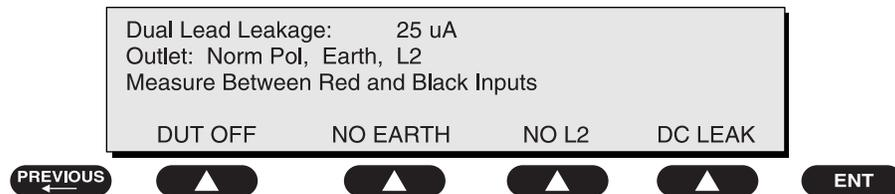
5. Measure point-to-point leakage between the RED and BLACK input jacks on the 601PRO.
