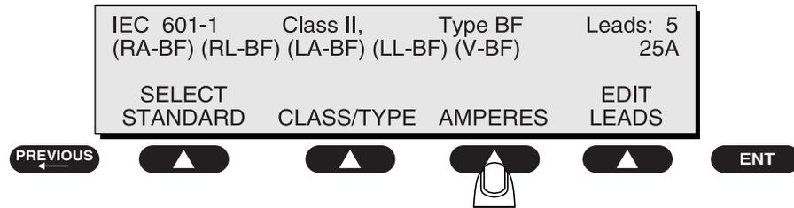
The test current displayed in the upper right corner will toggle between the available currents.
