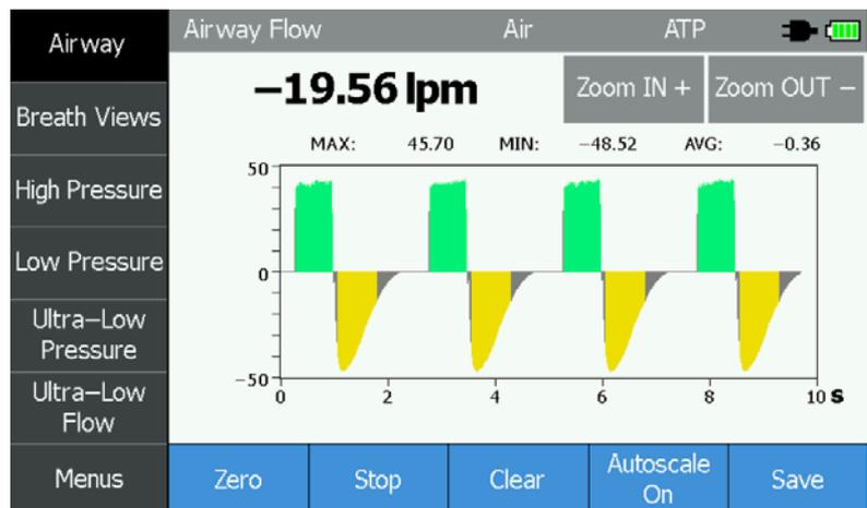
Figure 3. Airway graph of a typical ventilator with flow triggers set to 30 liters per minute
