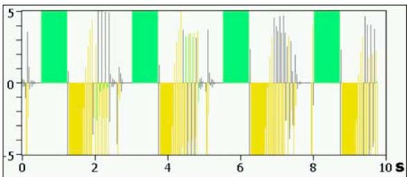
**Figure 8.** Airway flow zoomed in to +/-5 liters per minute with noisy flow on exhale
