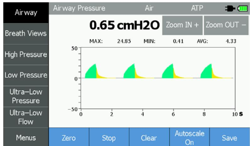
Figure 2. Airway Pressure graph of a typical ventilator
