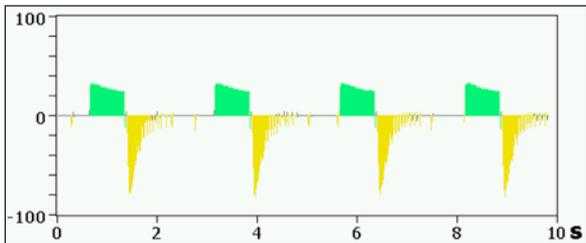
**Figure 7.** Airway flow with noisy flow on exhale due to PEEP setting
