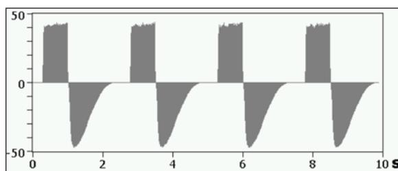
Figure 5. Airway graph with flow trigger set too high for both inspiration and expiration
