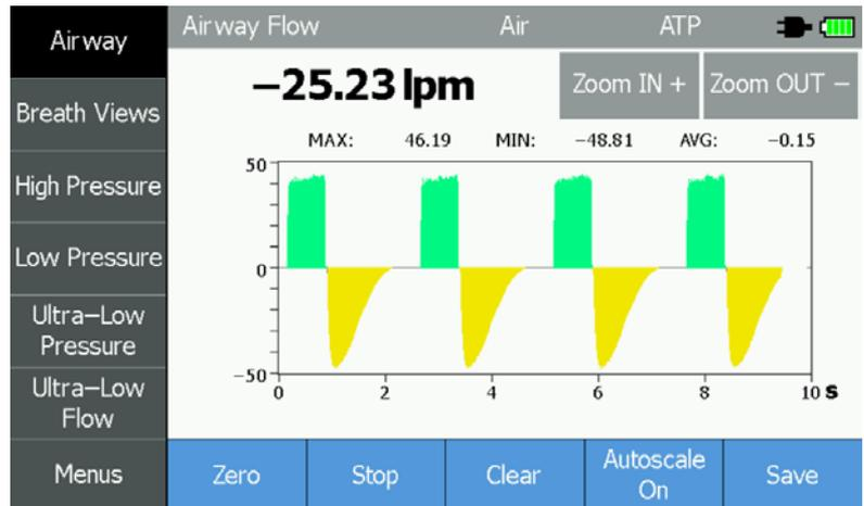
Figure 1. Airway Flow graph of a typical ventilator
