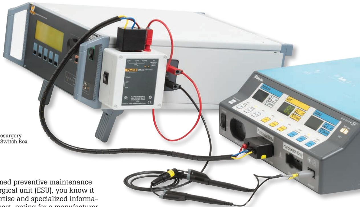
**Figure 1:** The QA-ES Electrosurgery Analyzer hooked up to The Switch Box and an Electrosurgery unit.
