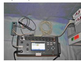
Setup for Philips Intellivue monitor.
