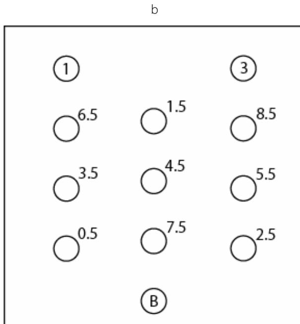
*Figure 1-2B. Test object numbered to indicate calibrated contrast at 80 kVp for the Half-Integer Phantom.*
