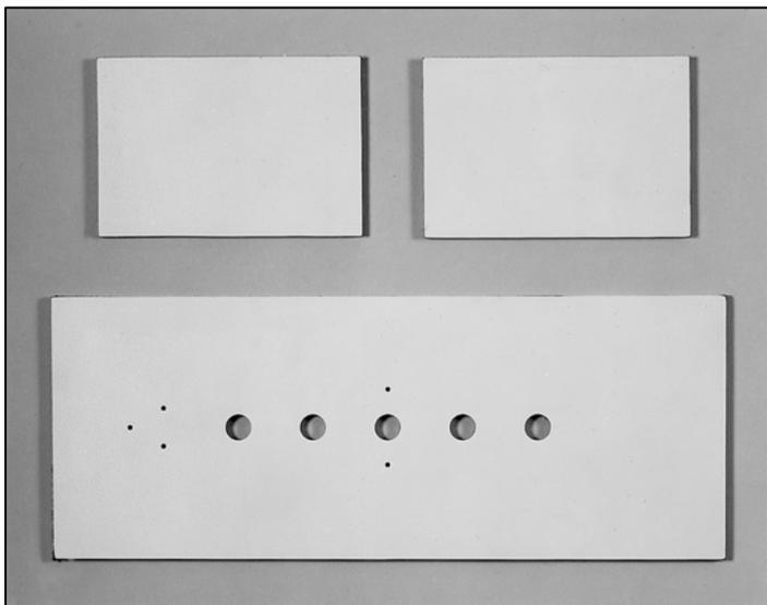
Figure 1-1. Model 07-644 Grid Alignment Test Tool, with Lead Blockers
