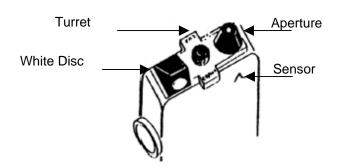
For lux measurements, the white disc is used. Place it over the light sensor. The location of the light sensor is designated by a mark  $(\land)$  on the instrument housing.
