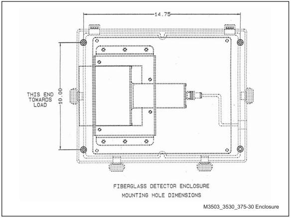
Figure 5. Detector Enclosure 385x106
