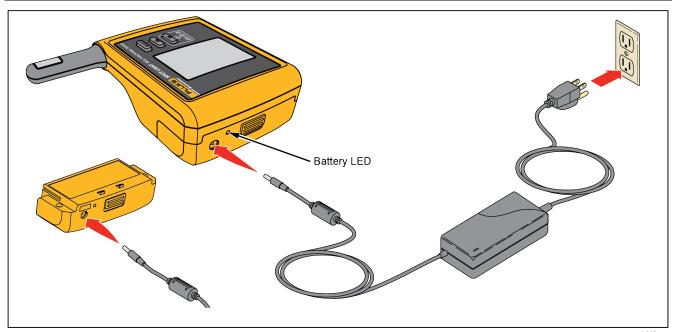
**Figure 6. External Battery Charger Connections**
