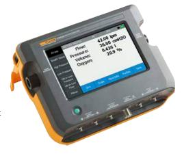
The VT900A features an external trigger input and special ultra-low flow and ultra-low pressure ports. These ultra-low flow and ultra-low pressure ports allow high accuracy for devices requiring crucial low volume and pressure testing such as anesthesia machines and flow meters. Designed and tested to world renown Molbloc-L calibration specifications ensures traceability to global regulatory standards with reliable measurements you can count on.
