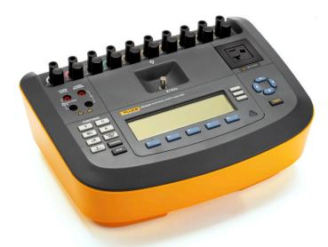
safety and basic tests on patient monitors can be performed with a single connection. When combined with optional Ansur computerbased software, the ESA620 allows for test procedure automation, the capture of results and comparison to standard limits, printed reports, and total digital data management.
