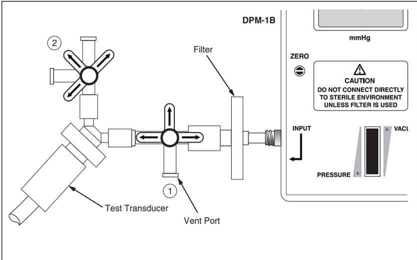
**Figure 4. DPM1B Configured to Apply Pressure to Transducer**
