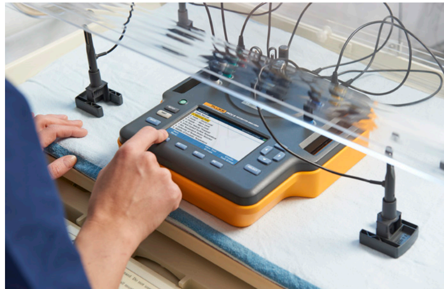
INCU II Incubator and Radiant Warmer Analyzer, testing an infant incubator.
