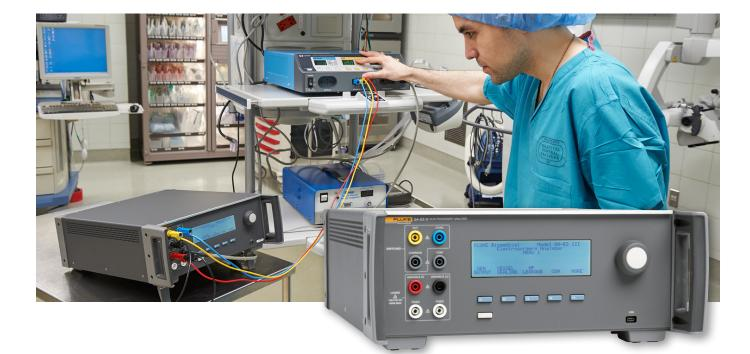
The QA-ES III Electrosurgical Analyzer simplifies testing to ensure the performance and safety of electrosurgical units. With generator output current accuracy as low as  $\pm$  2.5 %, the QA-ES III is capable of testing all modern high power electrosurgical units.
