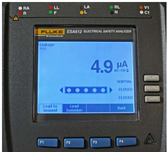
Example of a Patient (Applied Part to Ground) Leakage Current measurement using the ESA612 Electrical Safety Analyzer.
