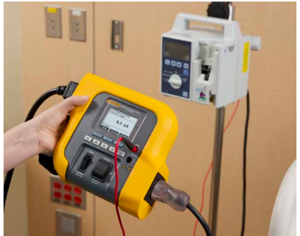
Example of a Chassis (Enclosure) Leakage Current Measurement using the ESA609 Electrical Safety Analyzer.
