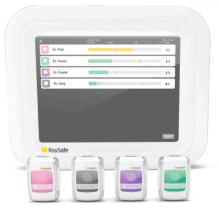
The fact is, when you know your exposure level you have a better chance of controlling it. One device that gives you this exposure insight is the RaySafe i3 personal dosimeter. RaySafe i3 provides you with constant, real-time radiation exposure information.
