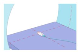
For kVp measurements, use an R/F sensor. Position it flat on the table and expose without rotation, using scout, tomogram or topogram mode. Use no or slowest table movement.
