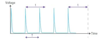
Stop delay setting longer than the time between pulses (t>T), will result in one long measurement. Note that you have to wait as long as the stop delay setting (t) after the last exposure before the measurement ends and values will be displayed.
