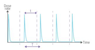
Stop delay setting shorter than the time between pulses (t < T), will result in many short measurements (one for each pulse).
