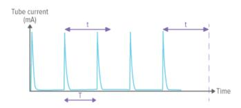
Stop delay setting longer than the time between pulses (t>T), will result in one long measurement. Note that you have to wait as long as the stop delay setting (t) after the last exposure before the measurement ends and values will be displayed.
