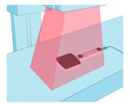
You can also use the sensor for low dose rate measurements, positioned centered in the X-ray field, with the dark side towards the radiation source.
