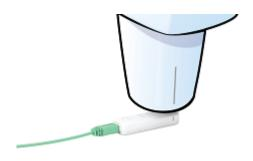
Place the connected sensor centered in the field with the crosshair towards the X-ray source. Make sure that the whole sensor rectangle is inside the direct beam.
