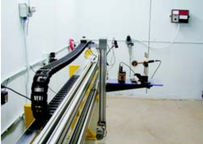
Dual-source range (500 mCi ^{137}\text{Cs} , 4 Ci ^{137}\text{Cs} )
