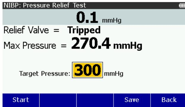
Figure 39. Pressure Relief Valve Test Results Screen
