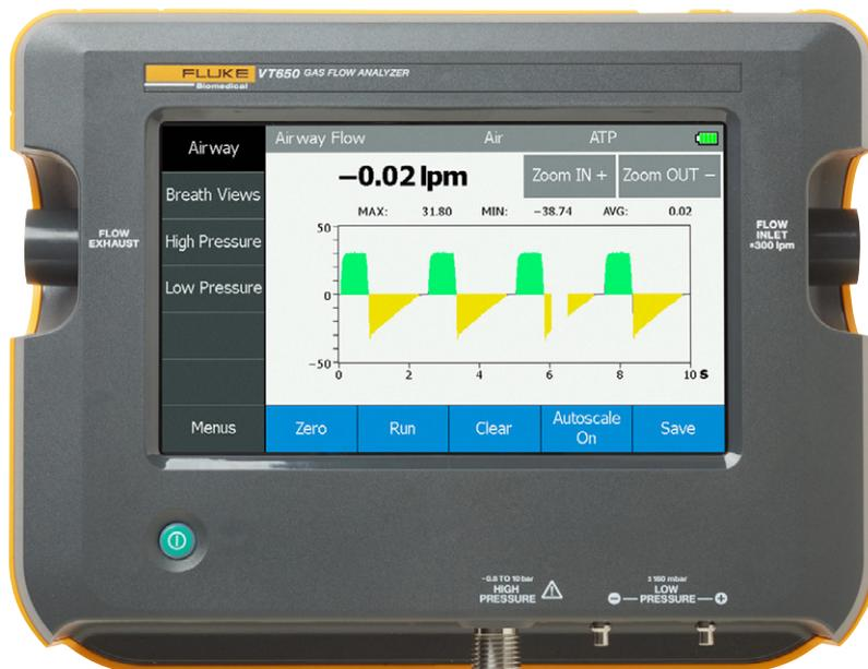
Full-range ±300 lpm air flow channel with built-in oxygen, humidity, and temperature measurements
