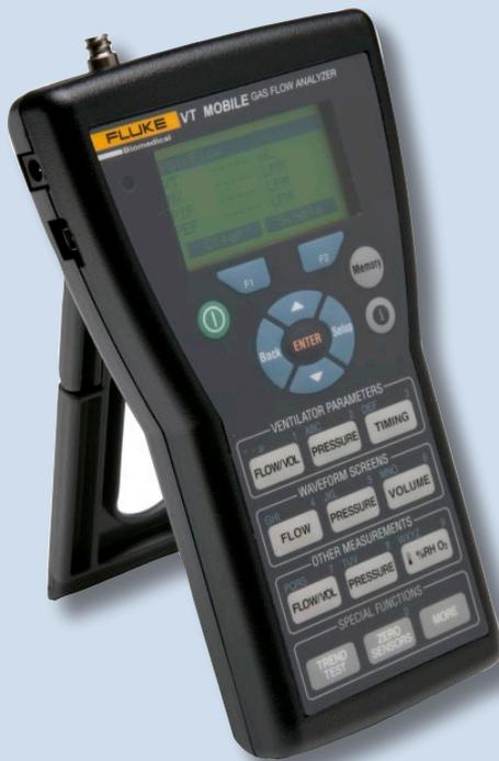
The VT Mobile is a compact and portable general purpose gas-flow analyzer designed to meet the needs of the traveling technician or engineer. This versatile tool evaluates performance of a wide variety of medical gas-flow/pressure devices and measures 16 ventilator parameters.
