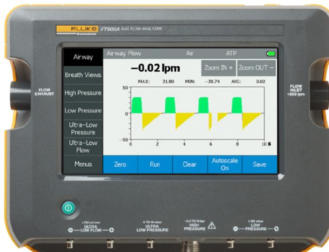
High and differential low pressure ports. All sensors have the best accuracies on the market, reliably calibrated using Fluke Molbloc-L system
